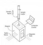
In this sketch, a sample is loaded into the top of the machine where there is a strong magnetic field. Radio waves are used to scan the sample and the results are fed to a computer. Credit: Jan Conroy/UC Davis
