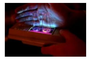
Organic phosphors developed at the University of Michigan could one day lead to cheaper organic light-emitting diodes. Here, they glow in blue and orange when triggered by ultraviolet light. Credit: Marcin Szczepanski, U-M College of Engineering
