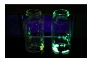
U-M researchers have developed pure organic phosphorescent crystals. Here, they glow yellow and green when triggered by ultraviolet light. Credit: Marcin Szczepanski, U-M College of Engineering
