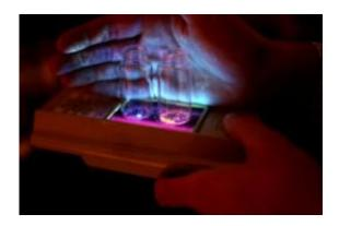
Organic phosphors developed at the University of Michigan could one day lead to cheaper organic light-emitting diodes. Here, they glow in blue and orange when triggered by ultraviolet light. Credit: Marcin Szczepanski, U-M College of Engineering
