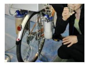
Japanese water purifier venture Nippon Basic displays a portable water purifying system "Cycloclean," powered by pedaling a bicycle to make a maximum of 5 liter of clean water in a minute at a technolocy fair in Tokyo. Nippon Basic Co. is gearing up for large-scale production in Bangladesh of the bicycle that can purify water at disaster zones or remote villages.
