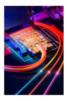
Light Peak module close-up with laser light added for illustration (actual infrared light is invisible to the eye).
