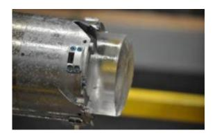
This is a section of an ice core coming out of the drill. Credit: Mark Twickler, University of New Hampshire
