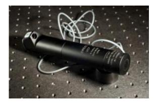
This prototype device developed by University of Rochester Professor of Optical Engineering Jannick Rolland can take high-resolution images under the skin's surface without removing the skin. Researchers say that in the future it may eliminate the need for many biopsies to detect skin cancer. Credit: J. Adam Fenster
