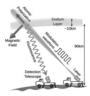
To measure the Earth's magnetic field, an orange laser beam is directed at a layer of sodium 90 kilometers above the Earth. The beam is pulsed at a rate determined by the local magnetic field in order to excite spin polarization of the sodium atoms. The fluorescent emission from the sodium, which depends on the spin polarization, is detected by a ground-based telescope and analyzed to determine the strength of the magnetic field. Credit: Dmitry Budker lab/UC Berkeley
