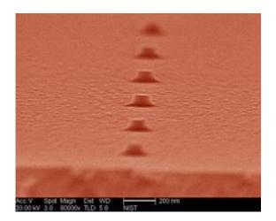
Colorized micrograph of quantum dots made using electron beam lithography and etching. This type of quantum dot can be shaped and positioned more reliably than dots made with conventional crystal growth methods. Credit: Verma/NIST
