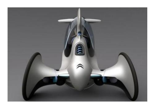
The <u>design</u> in low weight thanks to several features such as the shared suspension for both front wheels, the choice of a scratch resistant plastic in the vehicle canopy, and a rear wheel that doubles as a supportive structural element. Some choices, such as the plastic canopy are only possible because of the electric motors, which produce less vibrations than their gasoline and diesel fueled counterparts.
