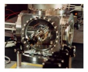
Ames engineers and scientists have equipped COSmIC with a custom-built timeof-flight mass spectrometer (TOFS), an ultra-sensitive device that detects the mass of matter at the molecular level. Credit: Farid Salama
