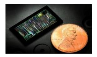
A completed photonic circuit measures less than an inch across. Credit: University of Washington
