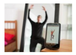
The electronic Fitness Assistant consists of a sensor suit that collects information about its wearer's movements and transmits results to a television, computer or smartphone. (© Fraunhofer IIS)
