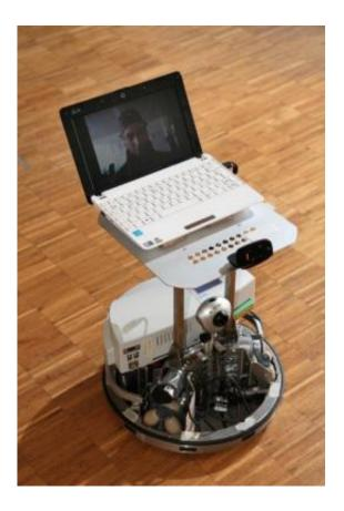
Robotino uses both "shared control" sensors and a recently developed system that uses probability theory to help users use the BCI for longer periods of time Credit: Alain Herzog / EPFL
