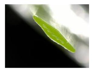
Cross-section of the fibre: It consists of five thin cores of polyamide and a sheath of polyethylene.
