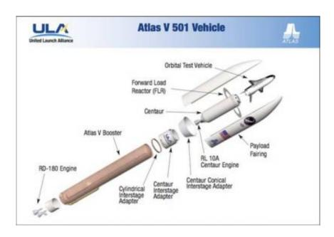
As seen in this diagram, the X-37B is encapsulated within the fairing of the Atlas
