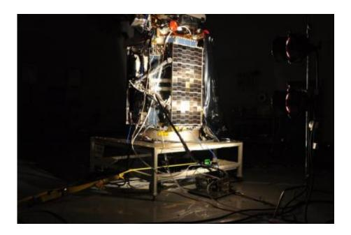
Inside the Astrotech Payload Processing Facility at Vandenberg Air Force Base, technicians illuminated Glory's solar arrays to confirm they were functioning properly following shipment from the factory in Virginia. Credit: NASA/Randy Beaudoin, VAFB
