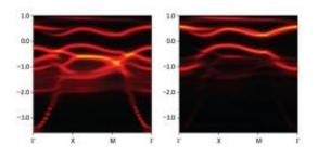
The energetic states of Sr2IrO4. The left panel shows the spectrum of all the computed electronic states. A gap in energy (y-axis) is clearly visible for electrons moving in all crystallographic directions (x-axis). The letters on the x-axis denote specific crystallographic directions. The right panel shows an isolation of the gap arising from states that form as a result of the spin-orbit interaction. Credit: Reproduced, with permission, from Ref. 1 2010 The American Physical Society
