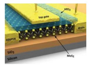
This is a digital model showing how molybdenite can be integrated into a transistor. Credit: Credit: EPFL
