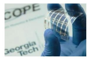
Researchers at Georgia Tech have demonstrated a new transistor for use on flexible plastic electronics, known as a top-gate organic field-effect transistor with a bilayer gate insulator. The transistor's properties give it incredible stability while exhibiting good performance. Credit: Canek Fuentes-Hernandez/Georgia Tech
