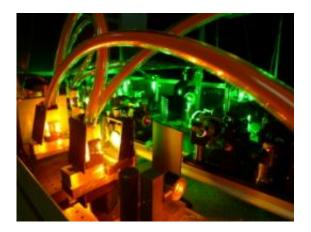
Resonance Ionization Laser Ion Source (RILIS) in action at ISOLDE. RILIS was instrumental in providing the pure beam necessary for the successful nuclear fission experiment.
