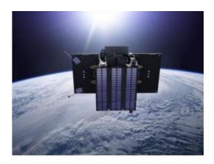
Proba-2 is flight-testing a total of 17 technology demonstrators for future ESA missions. It also serves as a scientific platform for solar and space weather observations. Credits: ESA/Pierre Carril
