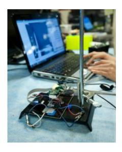
A small camera (white object with green circuit board on top), poised above the fluid chamber in the center of the black stand, transmits images of the paramecia as they swim about in response to changes in the polarity of an electrical field applied to the fluid chamber by the game player using a laptop computer.
