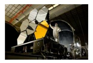
Ball Aerospace lead optical test engineer Dave Chaney inspects six primary mirror segments, critical elements of NASA's James Webb Space Telescope, prior to cryogenic testing in the X-ray & Cryogenic Facility at NASA's Marshall Space Flight Center in Huntsville, Ala. The James Webb Space Telescope will study the formation of the first stars and galaxies and shed new light on the evolution of the universe. Credit: NASA/MSFC/David Higginbotham
