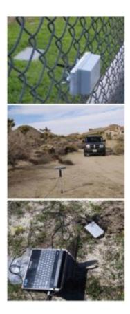
The USC Smart Fence system uses combined input from three sensors (top to bottom: motion, acoustic, and seismic), looking for spatiotemporal patterns of perimeter intrusion. Credit: USC Viterbi School of Engineering
