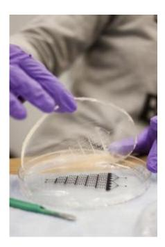
A student in the new Microfluidics Lab peels back the polymer, showing engraved channels, from an ink-transparency template. Credit: Eliza Grinnell, Harvard School of Engineering and Applied Sciences
