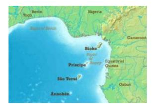
The source for one component of seismic noise appears to be the Bight of Bonny, a large, shallow bay off the west coast of Africa. When long-period water waves hit the continental shelf in the shallow bight, they are converted to seismic waves. Traditionally explorers defined a bight as a bay that could be sailed out of on a single tack in a square-rigged sailing vessel, regardless of the direction of the wind. This was possible only if the bay was slightly receding. Credit: WIKIPEDIA COMMONS
