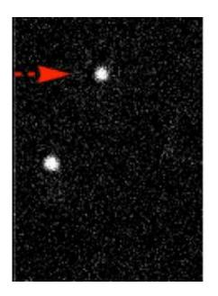
Electron micrograph showing multiple nano-sized electromagnetic hotspots on an aluminum film. Credit: courtesy of Xiang Zhang research group
