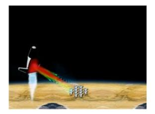
A conceptual microwave-propelled lightcraft receives microwave beams from an array of microwave sources on the ground. Credit: Kevin Parkin
