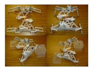
University of Vermont robotics expert Josh Bongard built this simple robot from Legos as proof of a complex idea, one that's teaching us about the interaction between brain and body. The Lego robot as well as simulated ones, evolve their body and their "brains" (or controller) together -- contributing to the faster development of more robust machines. Credit: Josh Bongard, University of Vermont
