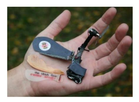
A natural samara is positioned next to the smallest and lightest robotic samara constructed to date. The wing of the vehicle is similar in size to a natural samara wing. Image credit: Ulrich, et al.
