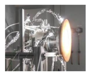
This is the ETH-Caltech solar reactor for producing H2 and CO from H2O and CO2 via the two-step thermochemical cycle with ceria redox reactions. Credit: Courtesy of ETH
