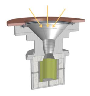
The ETH-Caltech solar reactor for producing H2 and CO from H2O and CO2 via the two-step thermochemical cycle with ceria redox reactions.
