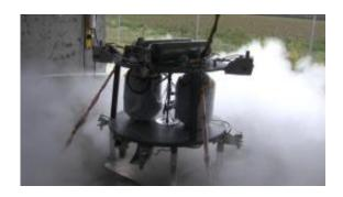
The robotic lander prototype's propulsion system, shown during a hot-fire test, consists of 12 small attitude control thrusters, three primary descent thrusters to control the vehicle's altitude, and one large "gravity-canceling" thruster which offsets a portion of the prototype's weight to simulate a lower gravity environment, like that of the moon and asteroids. Credit: Dynetics Corp.
