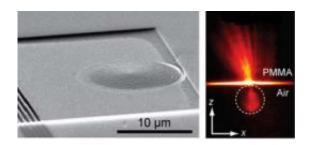
On the left is a scanning electron micrograph of a plasmonic Luneburg lens on a gold film. On the right, fluorescence imaging shows intensity of the SPPs propagated by the Luneburg lens (dotted circle). X marks the launching position of the electron beam and Z is the direction in which the SPPs propagate. Credit: Image courtesy of Zhang group
