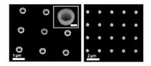
SEM images of nanoparticles fabricated for SERS by electron-beam lithography.
