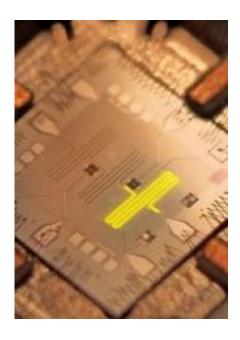
The photon shell game architecture: Two superconducting phase qubits (squares in the center of the image) are connected to three microwave resonators (three meander lines). Credit: Erik Lucero, Matteo Mariantoni, Dario Mariantoni
