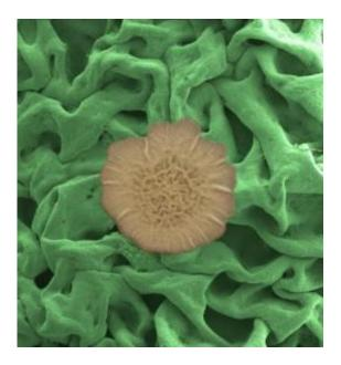
Slimy bacterial coatings known as biofilms (*Bacillus subtilis* colony superimposed at center) exhibit an unmatched ability to repel a wide range of liquids and even vapors. An electron microscope image shows the biofilm surface's resilient meshwork made from proteins and polysaccharides and assembled into a multiscale, hierarchical structure. Credit: Courtesy of the laboratory of Joanna Aizenberg, Harvard School of Engineering and Applied Sciences.
