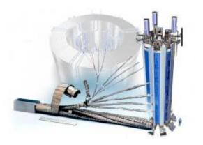
A schematic of ITER's central solenoid assembly.
