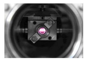
The circularly polarized ultraviolet light (UV-CPL) beam on the DESIRS beamline at the SOLEIL synchrotron facility, shown as it passes through a gas filter filled with xenon. Credit: Thomas Lannes
