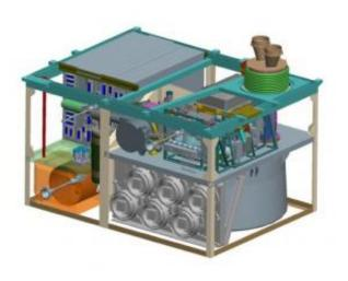
This schematic illustration shows major components of the microwave-oven-size instrument, which was installed into the mission's rover, Curiosity, in January 2011. Image Credit: NASA
