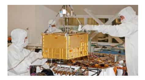
Techncians and engineers inside a clean room at NASA's Jet Propulsion Laboratory, Pasadena, Calif., prepare to install SAM into the mission's Mars rover, Curiosity. Image Credit: NASA/JPL-Caltech
