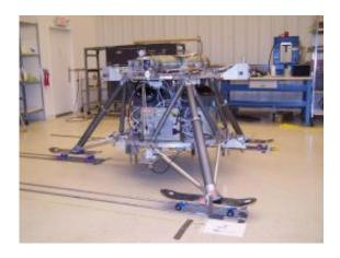
The robotic lander prototype was placed on modified skateboards and a customized track system as a low-cost solution to control movement during final testing of the prototype's sensors, onboard computer, and thrusters. (NASA/TBE)
