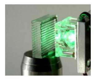
The luminous cube is the prototype of the new projector. Credit: Fraunhofer IOF
