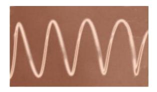
Zhu's research team has created the first coils of silicon nanowire on a substrate that can be stretched to more than double their original length, moving us closer to developing stretchable electronic devices. Credit: Yong Zhu, North Carolina State University
