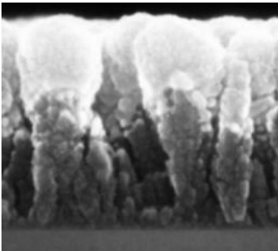
Researchers at Rensselaer Polytechnic Institute developed an entirely new type of nanomaterial that could enable the next generation of high-power rechargeable lithium (Li)-ion batteries for electric automobiles, laptop computers, mobile phones and other devices. The material, called a "nanoscoop"
