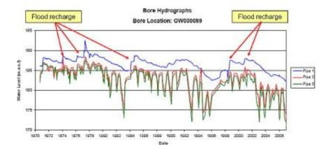
Reference bore at Wee Waa, New South Wales, showing response in water levels in response to floods between 1970 and 2006. Credit: The and Kelly (2010).
