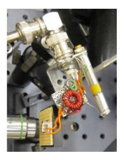
JILA instrument for generating terahertz radiation. Ultrafast pulses of nearinfrared laser light enter through the lens at left, striking a semiconductor wafer studded with electrodes (transparent square barely visible under the white box connected to orange wires) bathed in an oscillating electric field. The light dislodges electrons, which accelerate in the electric field and emit waves of terahertz radiation. At right is a close-up of the electron source. Credit: Zhang/JILA
