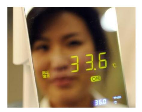
The world's first mirror thermometer, NEC Avio Infrared Technologies' "Thermo Mirror", is unveiled in Tokyo. The device measures the user's skin temperature without the need for physical contact, using a built-in infrared sensor.
