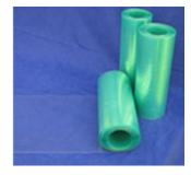
Fabricated rolls of moth-eye film; the rolls appear green due to the color of the protection film.
