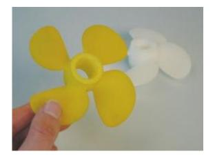
This propeller was dyed yellow in only five minutes at 90 degrees C and 200 bar. At this pressure, the yellow dye powder dissolved in the  $CO_2$  which transferred it into the plastic. Credit: Fraunhofer UMSICHT
