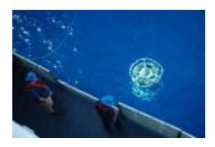
This shows the deployment of the CTD Rosette system for collecting water samples. Credit: Texas A&M University and NOAA
