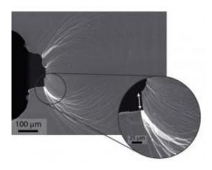
This micrograph of a deformed notch in palladium-based metallic glass shows extensive plastic shielding of an initially sharp crack. The inset is a magnified view of a shear offset (arrow) developed during plastic sliding before the crack opened. Credit: Image courtesy of Ritchie and Demetriou
