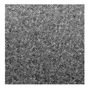
A transmission electron micrograph shows the amorphous structure of glassy palladium. (The area shown is 10 nm x 10 nm.) Credit: Caltech/Marios D. Demetriou
