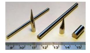
These are glassy palladium rods, with diameters ranging from 3 to 6 mm. Credit: Caltech/Marios D. Demetriou
